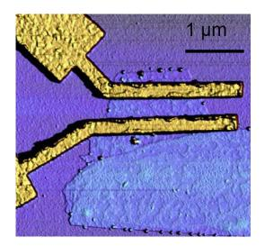
FIG. 2 Atomic force microscope image (false color) of a carbon monolayer covered by two superconducting Al electrodes. (Heersche et al., 2007)
